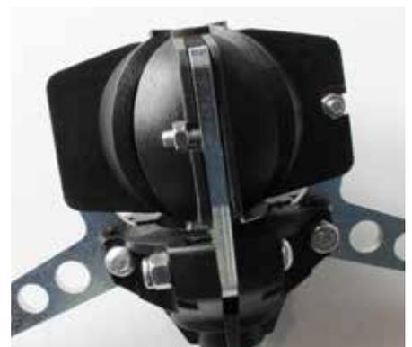
Change all four shells and check that when Ball Maker is closed all the shells all close perfectly without any gaps to make perfectly consistent groundbait balls.
