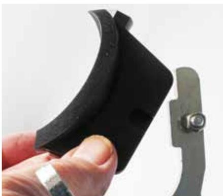
Shells can be changed easily, just undo nut and slide of shell and replace with different size shell making sure that it is pushed on as far as possible and then tighten nut.
